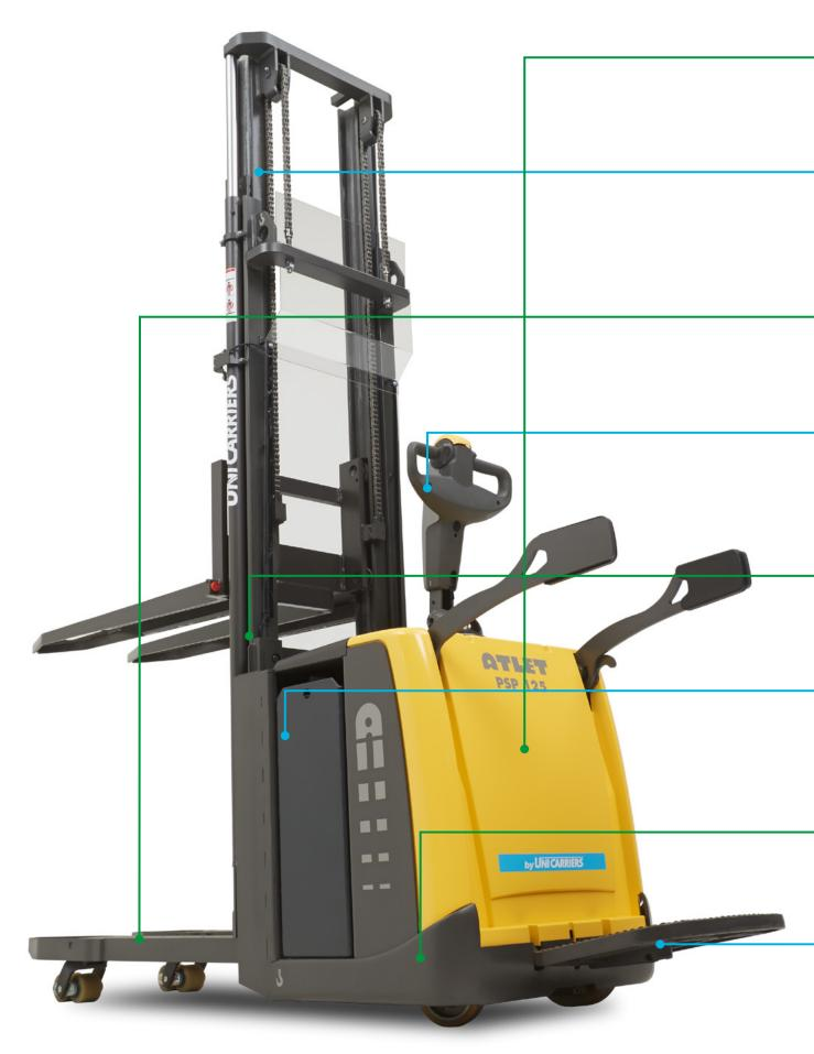
ProVision mast design with offcentre lift cylinder for optimised vision over forks.
