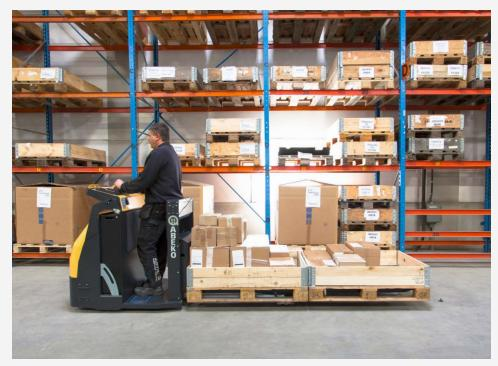
**Efficiency** The forklift can be equipped with several different fork lenghts for both one pallet but also with long forks to transport two pallets or three roll cages. The location of the wheels is adjusted for the handling required, at the same time the turning radius and stability is optimized according to the situation.
