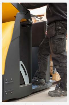
Step-in height What characterizes the MPL is the low step-in height and that one can easily go in and out of the truck on both sides. A essential part of an efficient order picking.
