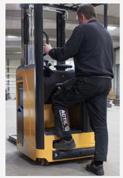
**Step-in** On SW 1350/1600 the step-in is only 230mm which helps the entry and exits from the forklift.
