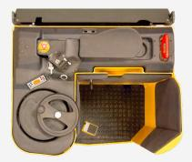
Workplace Here you stand at a 45 degree riding position for optimum driving forward/backward. The steering wheel and driving unit is stepless adjustable and vibration isolated to reduce strain in the hands and arms.
