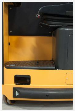
Floor adjustment To allow everyone to find an optimum driving position, the floor is both raise/lower and tilt adjustable. The low step-in height also makes getting in and out extra smooth.
