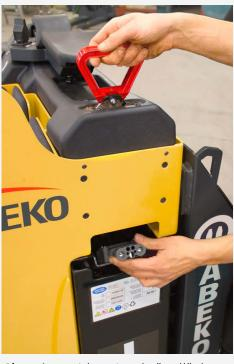
Charging With a simple "pull" the charging glove folds out to the side of the truck and it is easily connected to the charger.
