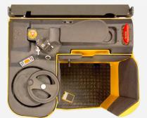
Workplace Here you stand at a 45 degree riding position for optimum driving forward/backward. The steering wheel and driving unit is stepless adjustable and vibration isolated to reduce strain in the hands and arms.
