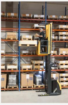
**OPL 10 3.0** Lifts up to 3000 mm, which means that you can effectively pick on several levels. With protective roof and gates orderpicking can be done safely.
