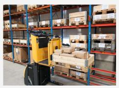
Workheight With ergolift the forks is adjustable to always be at a comfortable height. In it's up position the EUR-pallet is at a perfect height so that the driver easily can put down goods without strain.
