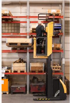
**OPL 10 2.1** Lift up to 2100 mm makes picking on several levels easy and with overhead guard and side gates it ´s safe.
