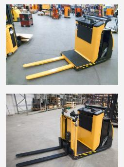
**Ergolift / fixed forks** All liftheights on our OPL can be equipped with either ergolift for an ergonomic picking or with fixed forks.
