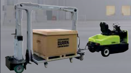
Tugger train with autonomous steering 1,600 kg
