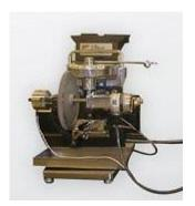
The Falex Pin & Vee Block Test Machine is a laboratory tool for evaluating wear, friction and extreme pressure properties of materials and lubricants. The equipment rotates a ¼ inch diameter test pin against two ½ inch diameter vee blocks. A four line contact is established as load is applied through a mechanical gage by a ratchet wheel and an eccentric arm. Standard Test Methods
