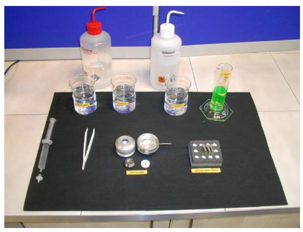
Attributes to perform a BOTD test: Cleaning fluids (aceton, white spirit and ethanol) Test fluid (ex. Diesel) Sample holder and cup assembly Ceramic balls and steel disks (or other materials)
