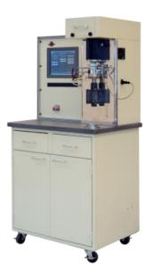
The Falex Four Ball Wear Test Machine is used to determine the relative wear-preventing properties of lubricating fluids and greases in sliding and rolling applications. Lubricants are compared using the average size of the scar diameters worn on the three lower clamped balls.
